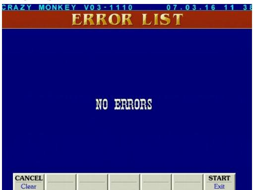
\*\* When System has NO ERRORS, press CANCEL for 5 seconds to INIT.
