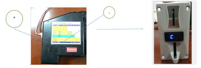
3: press "+"or "-" to adjust the coin quantity you want to use.. **Take 3 kinds of coin**  $\varphi$  **1.**  $\varphi$  **2.**  $\varphi$  **5as the example.** Adjust the number into "3" and press the set button to confirm.(number can be changed from 1-6 which mean one coin-6 kinds coin)
