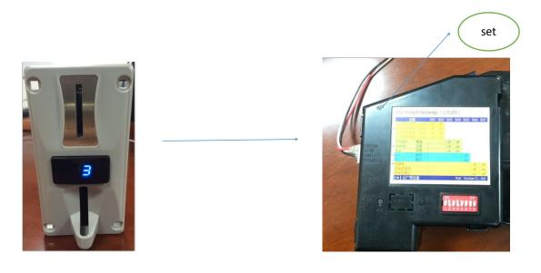
4: you can see the words:**P1**. It means the the pulse for the first coin. **You** can press "+" or "-" to adjust pulse you need. Take the 1 =1 pulse as the example.Adjust number into 1 and press set button to confirm.
