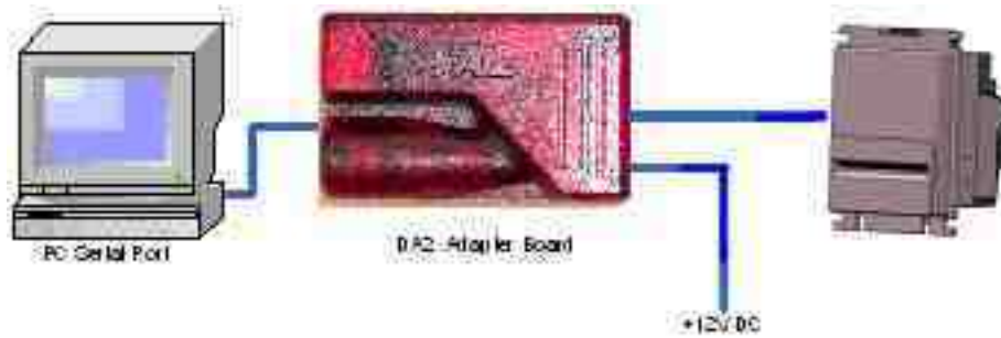
Figure 10 – Connecting DA2 to a BV20 and PC for upgrading Validator Programs
